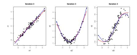
Red lines are smooth estimates of  $\phi_1$ ,  $\phi_2$ ,  $\phi_3$ , blue lines are the actual functions: the model  $y = x1 + x_2^2 + sin(x_3) + error$  was used to generate the data.
